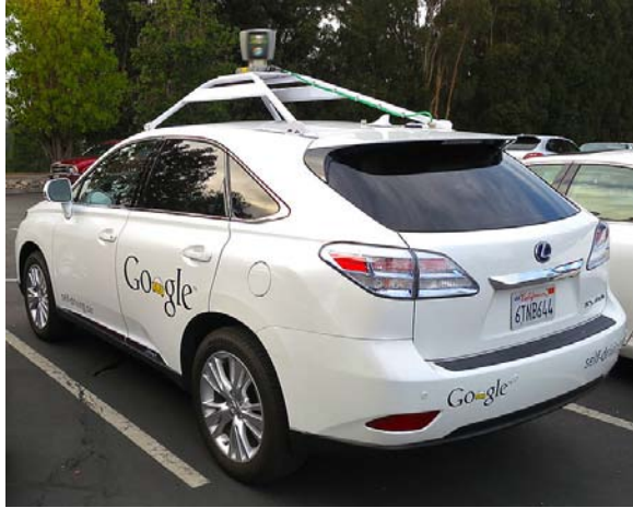
A conventional car (a Lexus RX 450h) modified by Google to become an autonomous car, with no human driver.
