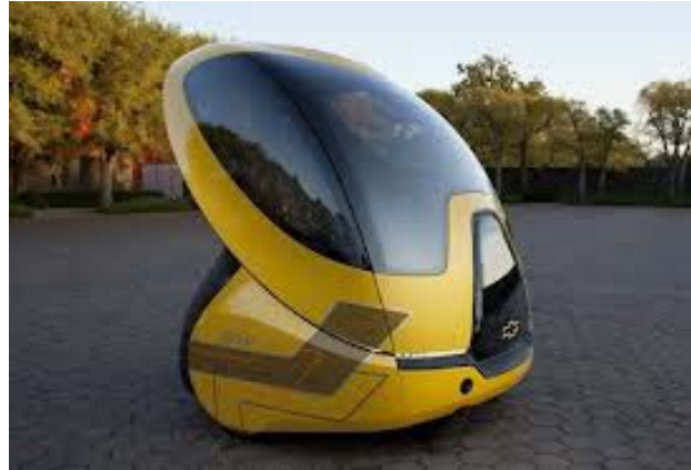
The Chevrolet EN-V (Electric Networked Vehicle) is a small-footprint 2-person vehicle that can be driven manually or autonomously.
